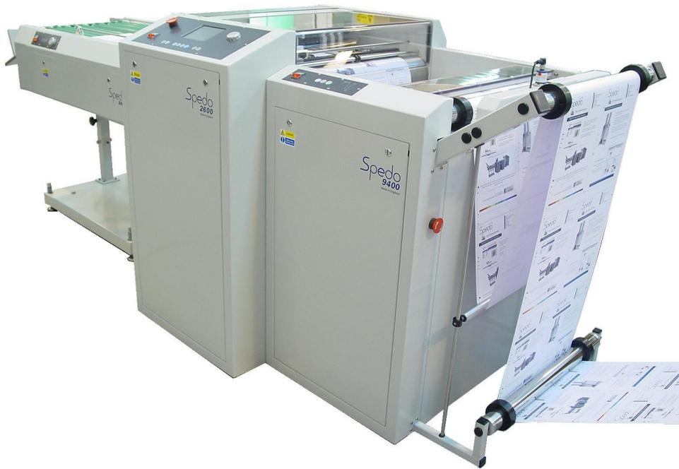
Easy optical mark set-up means that form registration can be done using any repeatable print area anywhere on the form, removing the need for the printer to add specific registration marks.
